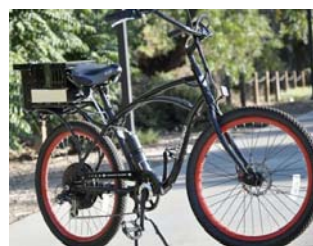
Figure 5. NaSi range extender powers a Pedego™ electric bike.
